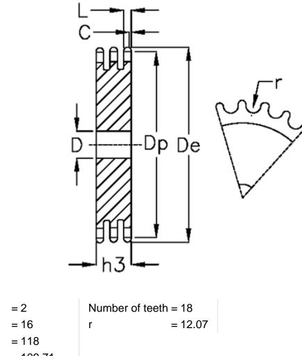
C = 2 D = 16 De = 118 Dp = 109.71 For chain size =  $3/4 \times 7/16$ For chain type = 12 B-3 h3 = 49.8 L = 10.8
